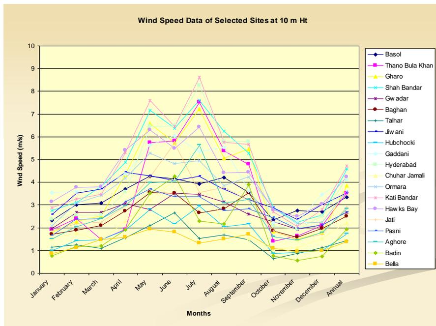
Figure 2: Wind data at 10 m height [5]
