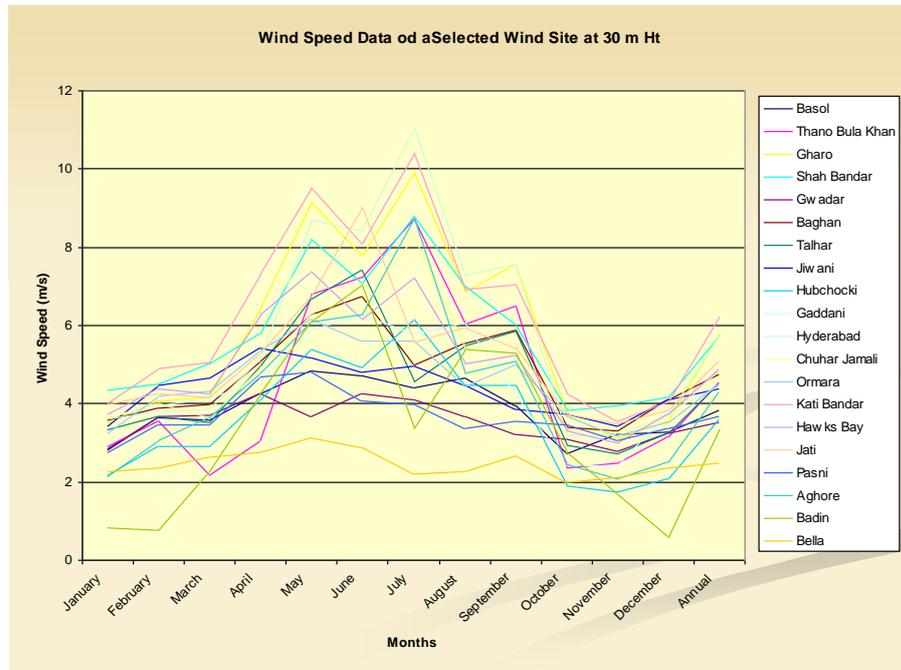
Figure 3: Wind data at 30 m height [5]
